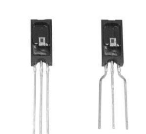
The HIH-3610 Series humidity sensor is designed specifically for high volume OEM (Original Equipment Manufacturer) users. Direct input to a controller or other device is made possible by this sensor's linear voltage output. With a typical current draw of only 200  $\mu$ A, the HIH-3610 Series is ideally suited for low drain, battery operated systems. Tight sensor interchangeability reduces or eliminates OEM production calibration costs. Individual sensor calibration data is available.
