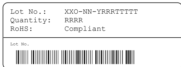
Figure 20: First label on reel: XX = Sensor Type (20 for SHT20), O = Output mode (D = Digital, P = PWM, S = SDM), NN = product revision no., Y = last digit of year, RRR = number of sensors on reel divided by 10 (200 for 2000 units), TTTTT = Traceability Code.
