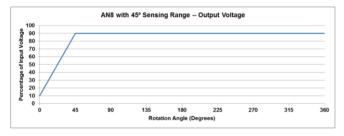
These charts show the output voltage as a percentage of the input voltage for a given angle of rotation. Example: 180° sensing range, magnet rotated 135°, output voltage will be 70% of input voltage (see dashed lines in graph above).
