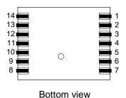
Fig. 2: Pin configuration of MS5536-60CPJU
