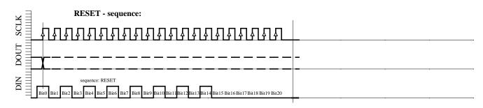
Fig. 6e: RESET sequence (21 bit)
