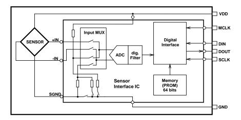
Fig. 1: Block diagram MS5536-60C
