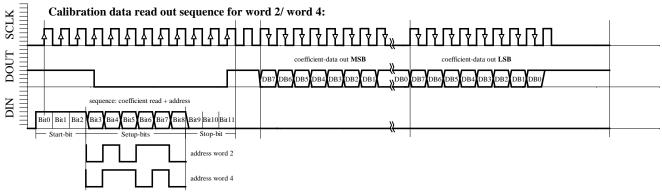
Fig. 6d: W2, W4 READING sequence
