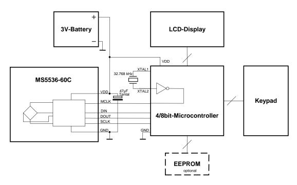
Fig. 7: Application example of the MS5536-60C for a battery powered device
