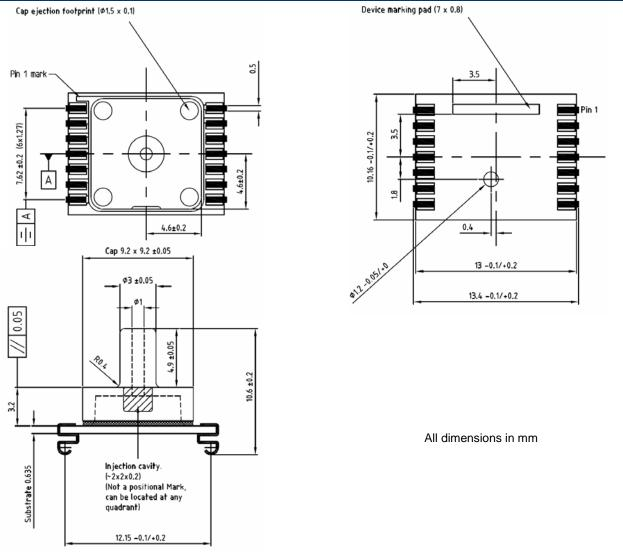
Fig. 8: Device package outlines of MS5536-60C-CPJU
