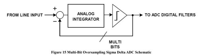
The use of multi-bit feedback and high oversampling rates reduces the effects of jitter and high frequency noise.
