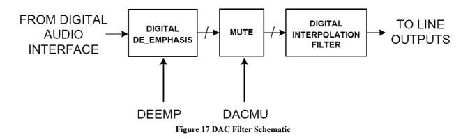
The DAC digital filter can apply digital de-emphasis under software control, as shown in Table 7.The DAC can also perform a soft mute where the audio data is digitally brought to a mute level. This removes any abrupt step changes in the audio that might otherwise result in audible clicks in the audio outputs.
