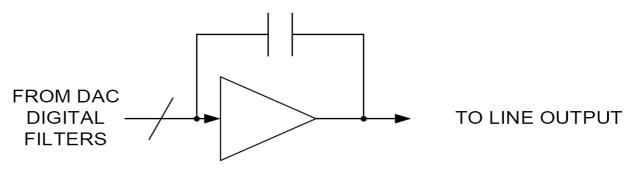
Figure 18 Multi-Bit Oversampling Sigma Delta Schematic
