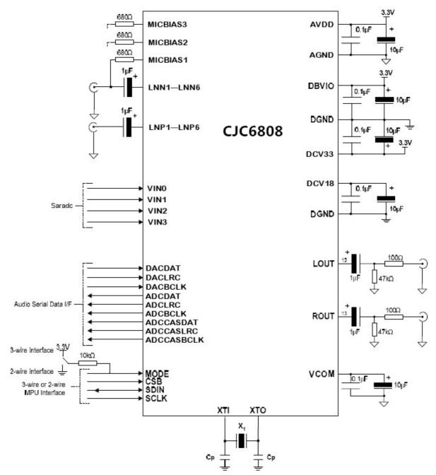
Figure 57 External Components Diagram
