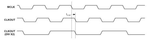
Figure 2 Clock Out Timing Requirements
