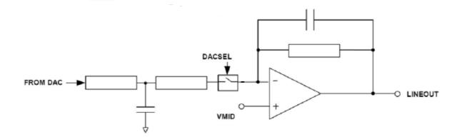
Figure 19 Line Output Schematic
