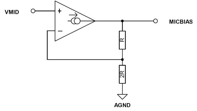
**Figure 14 Microphone Bias Schematic**
