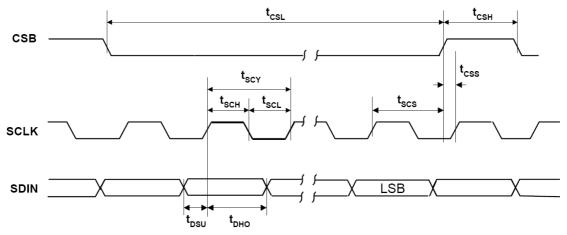
Figure 7 Program Register Input Timing - 3-Wire MPU Serial Control Mode
