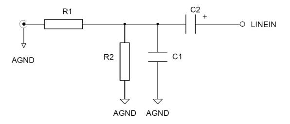
Figure 11 Line Input Application Drawing
