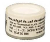
This sensor is specifically designed for percent oxygen analyzers offered by Advanced Instruments Inc.
