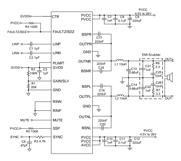
Fig2. Typical PBTL Mode Applications
