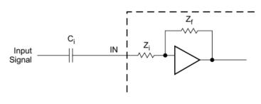
Figure 25. Input Impedance
