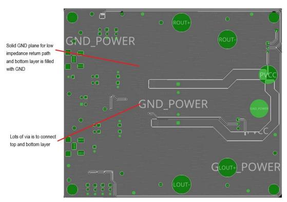
Figure31. Layout Example Bottom
