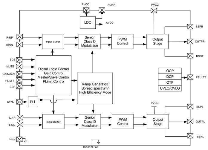
Fig5. iML6603 Functional Block Diagram
