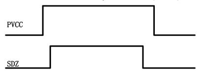
Fig26. Timing Requirement for SDZ and PVCC
