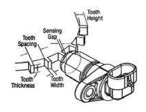
For best results, we recommend targets made from low carbon cold rolled steel. Other factors that influence sensor performance include gear tooth height and width, space between the teeth, shape of the teeth and thickness of the target. As a general guideline, consider a target with minimum parameters as shown below. Note that smaller dimensions may work, but testing for the application is required.
