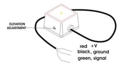
The 110-WS-16BP Barometric Pressure Sensor uses a piezoresistive sensing element which responds to changes in barometric pressure with a corresponding change in resistance. This resistance is converted to a voltage from which a microprocessor (or another data processor) calculates the barometric pressure at the elevation where the barometer is located.
