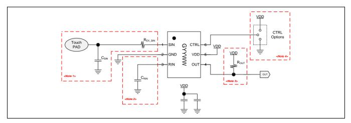
**NOTE:**  $R_{EXT\_SIN} = 200 \Omega$ ,  $C_{SIN} = 1pF$ ,  $C_{RIN} = 1pF$  (recommend)
