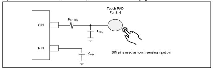
Implementation circuit for SIN pins and RIN pin is shown in the following figure.
