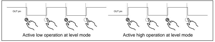
The OUT pin waveform for level and toggle operation
