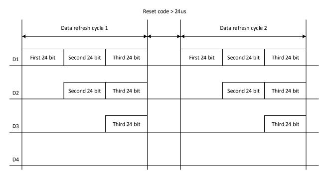
Figure 2. Data Transmission Format
