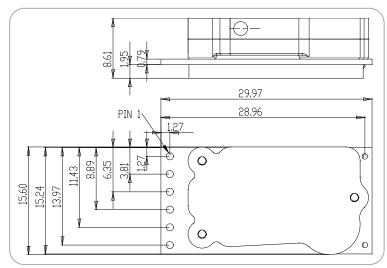
All dimensions in millimeters (mm)
