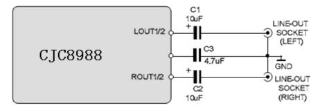
Figure 44 Recommended Circuit for Line Output
