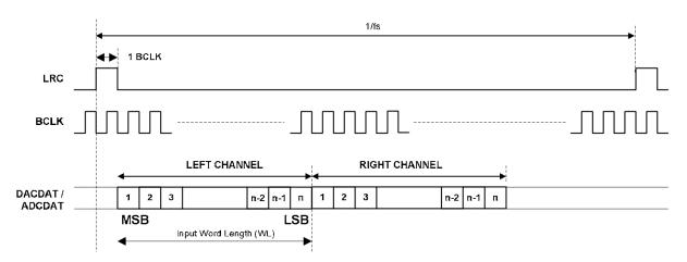
Figure 14 DSP/PCM Mode Audio Interface (mode A, LRP=0, Master)
