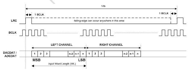
Figure 16 DSP/PCM Mode Audio Interface (mode A, LRP=0, Slave)
