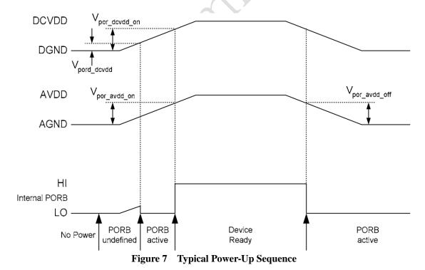
Figure 7 shows a typical power-up sequence. When DCVDD and AVDD rise above the minimum thresholds, Vpord\_dcvdd and Vpord\_avdd, there is enough voltage for the circuit to guarantee the Power on Reset is asserted low and the chip is held in reset. In this condition, all writes to the control interface are ignored. When DCVDD rises to Vpor\_dcvdd\_on and AVDD rises to Vpor\_avdd\_on, PORB is released high and all registers
