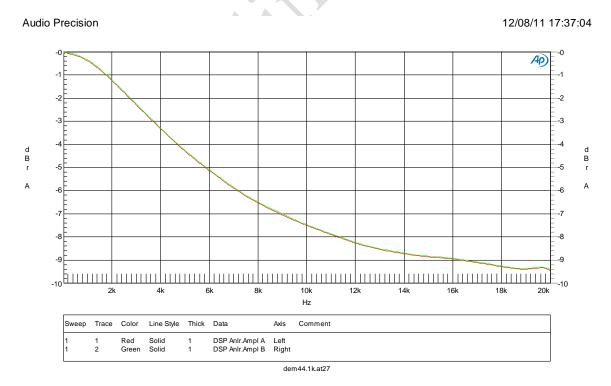
Figure 22 De-emphasis Frequency Response (44.1kHz)
