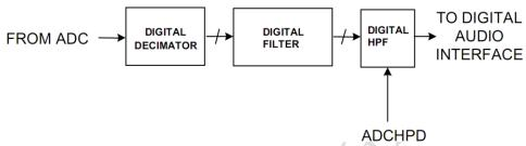
Figure 8 ADC Digital Filter
