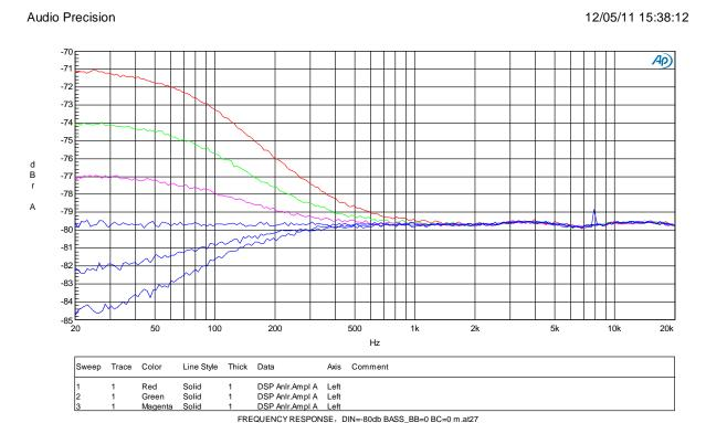
Figure 36 FREQUENCY RESPONSE, DIN=-80db BASS\_BB=0 BC=0
