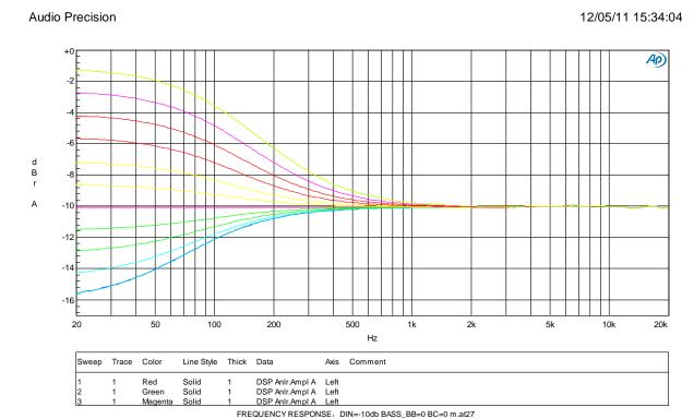
Figure 32 FREQUENCY RESPONSE, DIN=-10db BASS\_BB=0 BC=0
