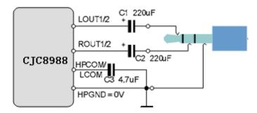
Figure 43 Recommended Headphone Output Configurations
