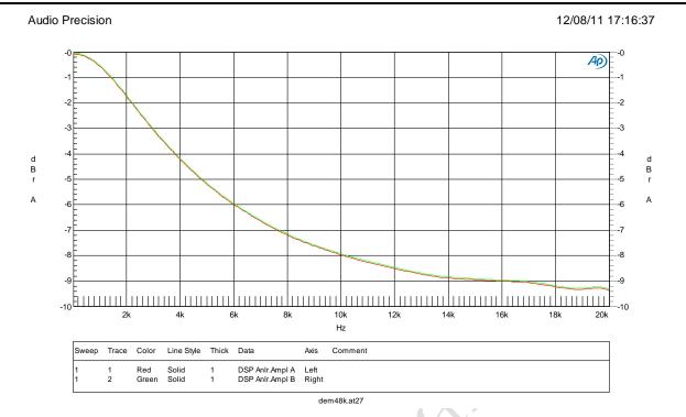
Figure 23 De-emphasis Frequency Response (48kHz)
