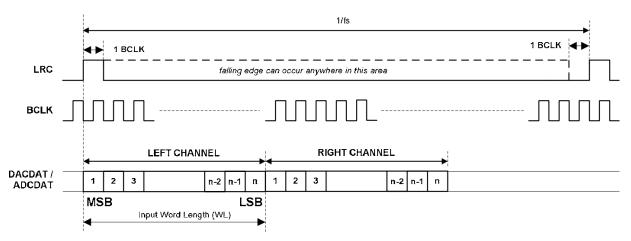
Figure 17 DSP/PCM Mode Audio Interface (mode B, LRP=0, Slave)
