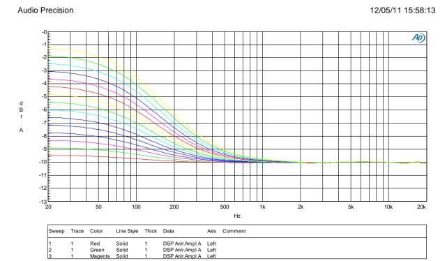
Figure 34 FREQUENCY RESPONSE, DIN=-10db BASS\_BB=1 BC=0
