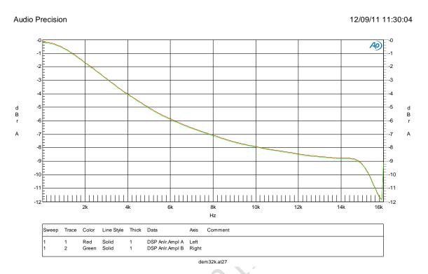
Figure 21 De-emphasis Frequency Response (32kHz)
